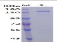
Biotinylated ACE2-hFc, Avitag on SDS-PAGE under reducing (R) condition. The gel was stained overnight with Coomassie Blue. The purity of the protein is greater than 95%.
