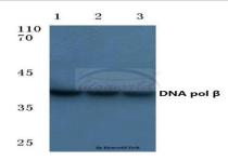
Western blot (WB) analysis of DNA pol  $\beta$  (Q324) polyclonal antibody at 1:500 dilution
